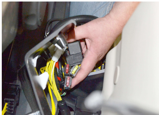
Trailer Plug Fuses (Located behind plastic panel on pillar behind passenger seat)
