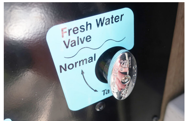
Fresh Water Valve (Shown in the open position. Turn valves to close). This is on the T36A -Typical View
