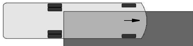
Weighing Right Front Corner
