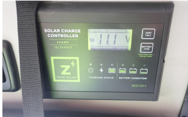
Solar Charge Controller (Located near the Systems Monitor Panel) -Typical View
