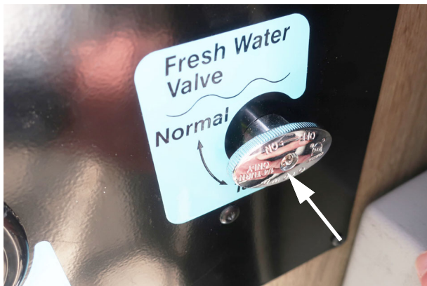
Fresh Water drain Valve (Located on Water Center Panel shown in the closed position for the T36A). -Typical View
