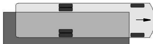
Weighing Right Rear Corner
