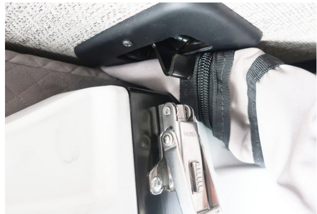
Travel latch shown unlatched and folded out of the way. -Typical View
