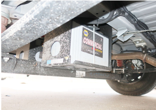
House Battery Access (Located in front of the rear tires) - Remove bolts from battery retainer to remove house battery
