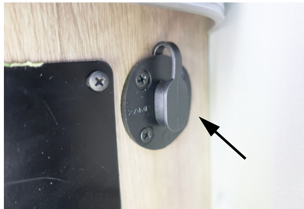
Single Solar Port (Located inside the passenger rear door above the Water Center Panel) -Typical View
