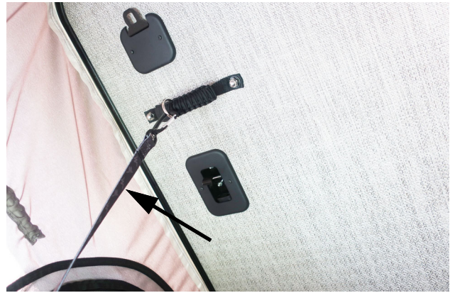
The included pull straps are used to assist in pulling the pop-top back down. Those are attached by a d-ring to both pop-top handles. -Typical View
