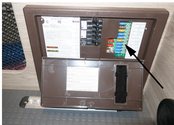
House 12-Volt Fuses (Located on the drivers side panel below the folding bed.) -Typical View
